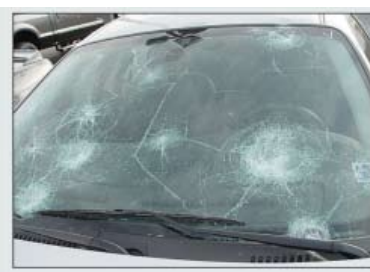
Laminated glass adheres to the inner plastic sheet, preventing shatter
